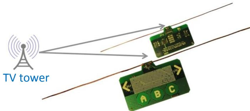
TV tower powered battery-less devices
