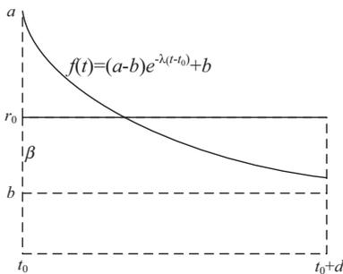
Fig. 5. The rate function follows an exponential decay, starts at  $a$ , goes down below  $r_0$  but guarantees a minimum rate  $b$ .
