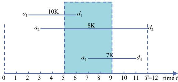
**Fig. 2.** An illustration of remaining packets and available epochs after applying the first iteration by *DIF-Policy* on the packet set of Fig. 1. Epochs in shaded area are not available for remaining packets.
